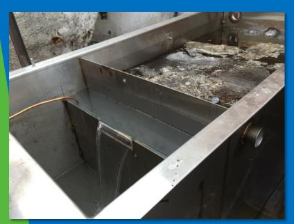
Oil water separators (OWS) are effective, but they do require periodic maintenance to perform as designed. Over time, solids accumulate in the chambers thereby reducing the capacity, flow, and effectiveness of the separator itself. If these solids are not periodically vacuumed out and disposed of, a bypass can occur which will allow oil to be discharged instead of cleaned effluent. This can lead to a permit violation and expensive compliance issues.
